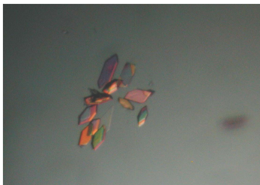
Figure 2 Typical crystals of the dodecamer d(CGCGAATT*CGCG) (* indicates inserted ribose) obtained by hanging-drop vapour diffusion. The largest crystal is 0.20 mm in length.
